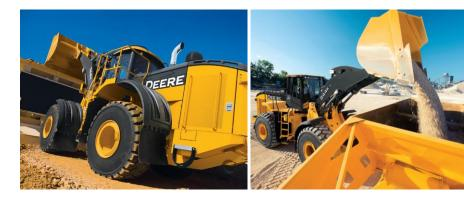
Programmable clutch cutoff increases productivity in all kinds of conditions. Engaging the brakes disconnects the transmission while maintaining high engine speed. For smooth dumps, fast cycles, and no machine rollback. Boom-height kick-out sets maximum desired dump height, while returnto-carry determines lowered-boom position. Use these two K-Series advantages to speed production in repetitive loading applications.
