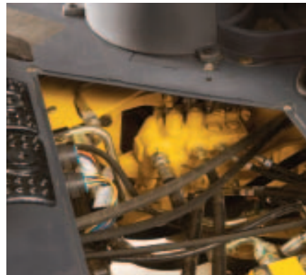
Split floor mats and a large removable panel provide convenient, top-side access to internal components.
