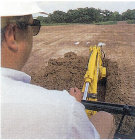
Boom starts wide at the base and narrows to 9 inches through the line-of-sight. Unlike the large "dorsal fin" on other excavator-style booms, the 310SE's compact cylinders share a single-pin attaching point that doesn't impair side-swing visibility, either.
