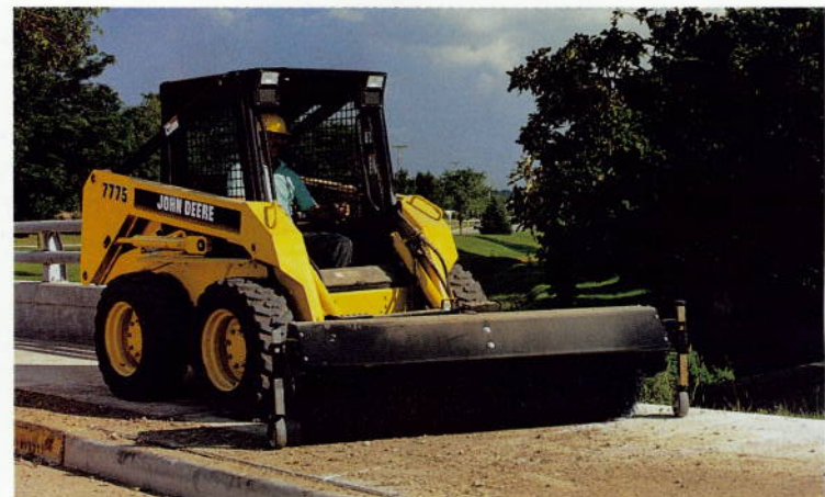
ANGLE BROOM. Adjustable twin casters and oscillating frame follow ground contours. Poly/steel, 22-in. diameter. Clears 63.5 to 70 in. path. Fits 4475, 6675, 7775 Skid-Steers.
