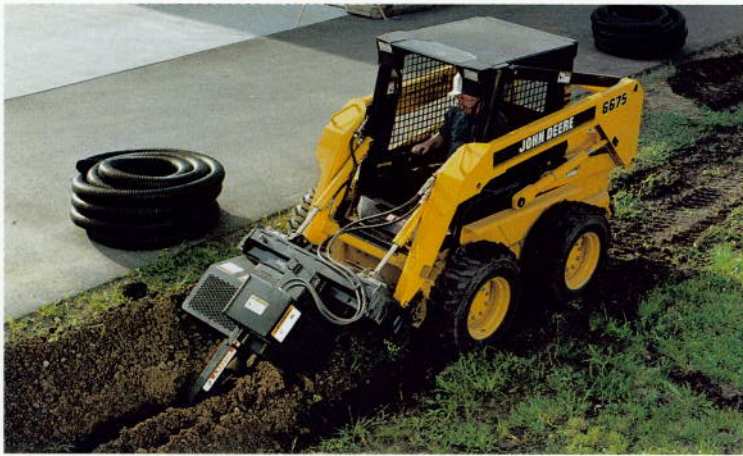
TRENCHERS. Great for laying wire or pipe. Two sizes, 3- or 4-ft. boom. Double standard, anti-backflex, 5-1/2 to 6-in. adjustable chain. Adjustable, replaceable spoil auger. Fit all but 3375.
