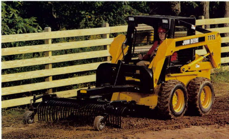
LANDSCAPE RAKES. Heavy-duty 6- and 7-ft. sizes. Pivot 180 degrees for push or pull operations. Flip-down grader blade, adjustable wheels. Fit 4475, 6675 and 7775 Skid-Steers.
