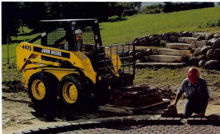
PALLET FORKS. Load pipe, conduit, stone and other materials. Three sizes—36, 42, and 48 inches long, with variable fork spacing. Fit 4475, 6675 and 7775.
