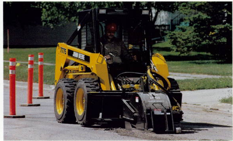
COLD PLANER. Quickly cuts up damaged concrete or asphalt. Pivoting center drum; hydraulic depth, tilt and side shift. Requires optional hi-flow hydraulic kit. Fits 6675 and 7775 Skid-Steers.
