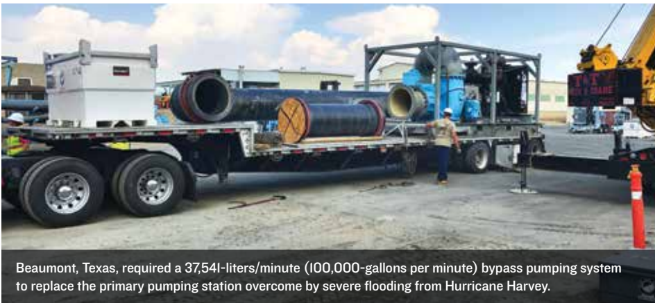
After Hurricane Harvey, Rain for Rent of Bakersfield, California, delivered and installed DV600c pumps powered by PowerTech Plus 13.5L engines in Beaumont, Texas.
