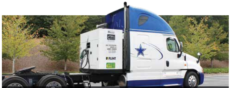
Mounted behind the cab, the 60-kWe John Deere-powered generator powers the lights and air conditioning, as well as the hydraulically powered awning and slide-outs.
