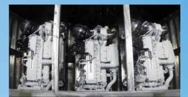
Three John Deere 9.0L engines power HamiltonJet 322 waterjets through a ZF transmission with a 1:1 gear ratio.
