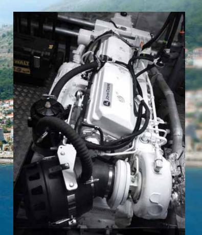
Twin John Deere 13.5L engines propel *Swallow* through a Dong gearbox with a 5.04:1 gear ratio.
