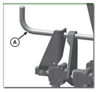
Verify single-point depth control is disengaged to allow TruSet™ depth control system to function properly. Rotate the crank (A) fully clockwise.
