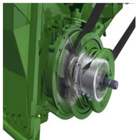
Dry Stalk Conditions – Operate the corn head at the higher variable speed drive 510- 640RPM (without excessive butt shelling). No faster than 3<sup>rd</sup> gear (620-640) on a 5 Speed drive. The fast corn head drive speeds allow the stalk rolls to pull more trash down and cushion the ears to minimize butt shelling.
