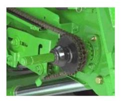
Feed Accelerator Speed Slow side speed - 430 rpm Inner Large Diameter
