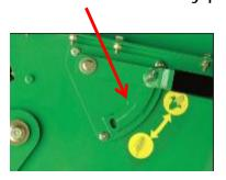
Chopper speed on high (pull knob out). Also engage knife bank depending on preferred residue size.
