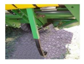
Reel Position & Speed: Run the reel up and back to reduce pod shatter. In shatter resistant verieties, run the reel just into the crop to assist feeding. Reel speed should be matched to ground speed, or approximately 10% faster then ground speed to correctly flow material.
