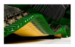
Automatic Header Height Sensing – Needs to be calibrated before harvest begins to ensure a good clean cut.
