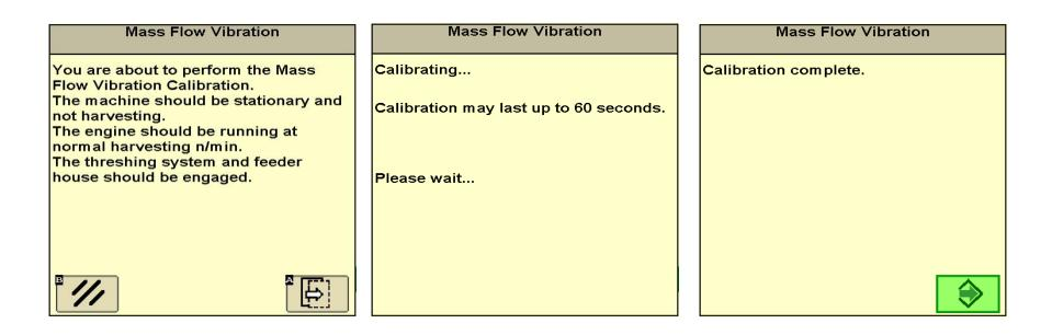
4. Follow the instructions in the calibration. Engage the header and separator, with the header in the harvesting position take the engine speed to high idle, be sure the header is not resting on the ground and the grain tank is empty.
