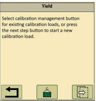
**4.** Select the "next" button to begin the calibration, be sure the grain tank is empty.
