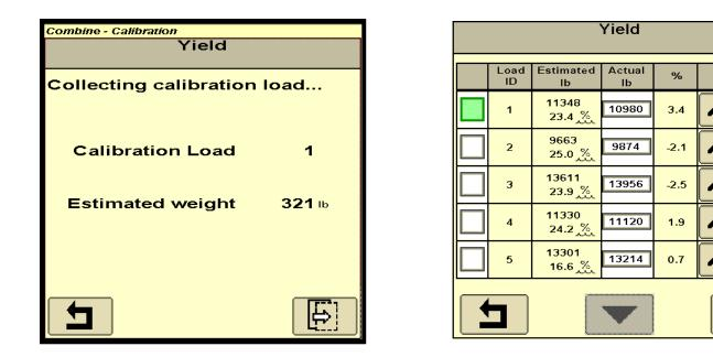
6. Unload and record the actual scaled weight. Select the "next" button and enter the "Actual" scale weight in the numerical box.
