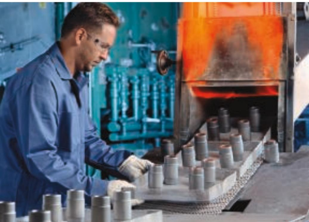
**In a patented process, alloy powders, atmospherics, and 2,000-deg. heat fuse the SC-2 coating fast to the part.**
