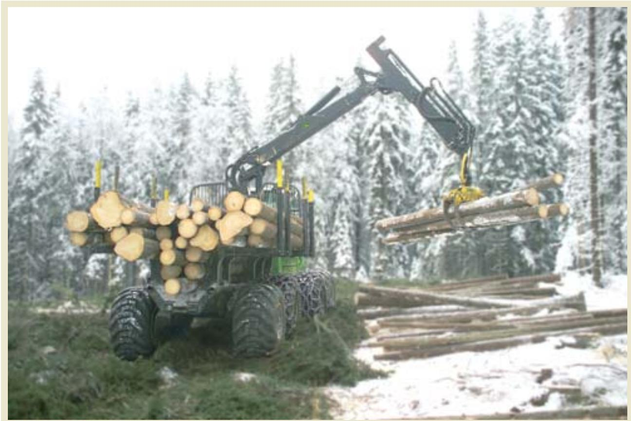
The strongly built long-reaching booms are positioned at an appropriate distance almost parallel to the operator's field of vision. This allows for smooth and natural controlling of movements. Optional equipment include hydraulic dampening of the slew and lifting motions and an ASF - function for the boom of the 810D, which adjusts the position of the boom and holds the grapple still above the load while the machine is turning.
