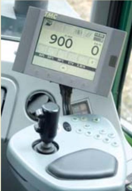
The Timbermatic 700 system is available as an alternative to the TMC system. The Timbermatic 700 creates a tele-communications link between the harvester and the forwarder, generating advantages through providing information on the location of logs produced by the harvester. The large colour display provides the operator with the tools of the Windows environment from email to maps and GPS software.
