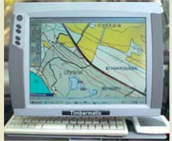
The Timbermatic 700 and the TMC improve overall productivity and allow for easy use of the latest monitoring tools, such as the boom scale and the reverse camera. The sensors and software of the optional boom scale measure the weight of the load and the logs. This allows for efficient use of the load space: the loads remain a suitable size and forwarding is safe and fast. The self-learning calibration function of the scales increases the reliability of the system.
