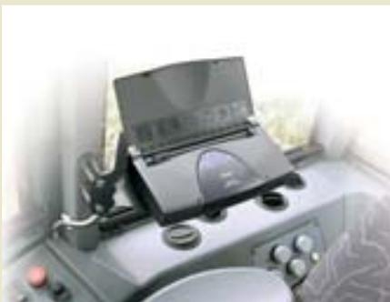
The software features a versatile fault diagnostics function and the system issues reminders of scheduled maintenance services. The reports produced by the Timbermatic 700 can also be printed out using an A4 size colour printer.
