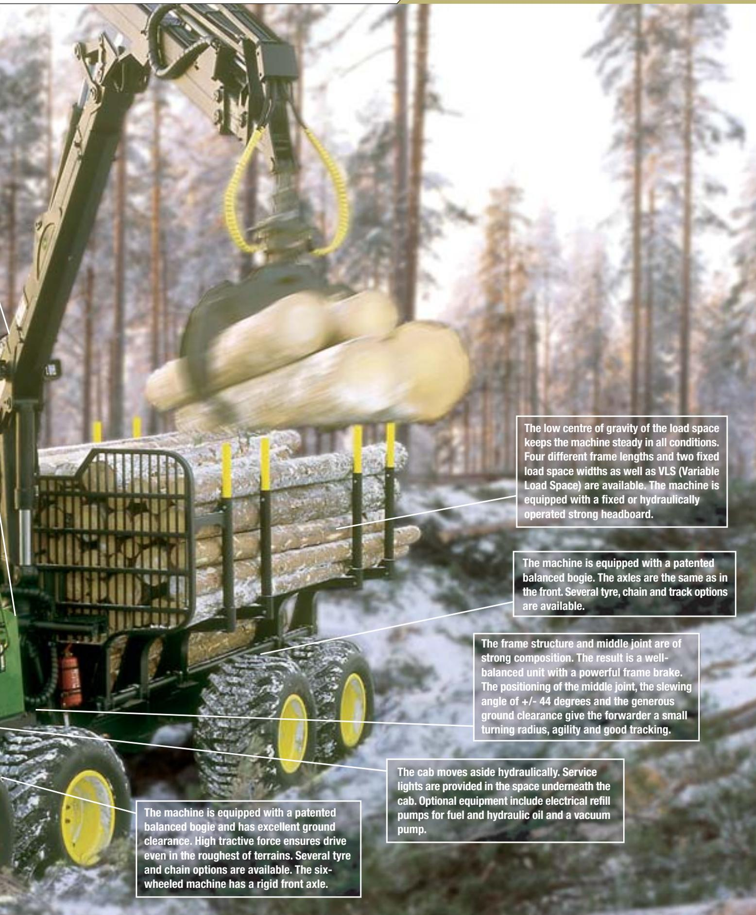
The low centre of gravity of the load space keeps the machine steady in all conditions. Four different frame lengths and two fixed load space widths as well as VLS (Variable Load Space) are available. The machine is equipped with a fixed or hydraulically operated strong headboard.
