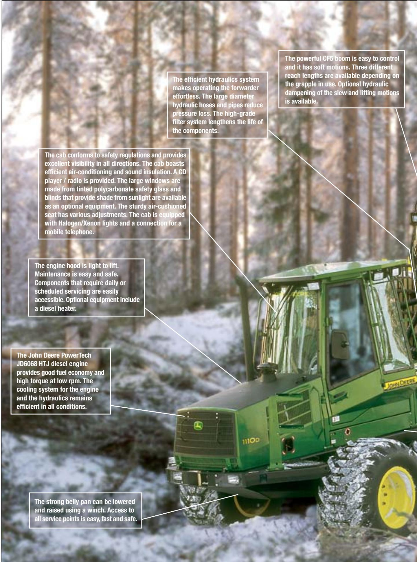
The efficient hydraulics system makes operating the forwarder effortless. The large diameter hydraulic hoses and pipes reduce pressure loss. The high-grade filter system lengthens the life of the components.
