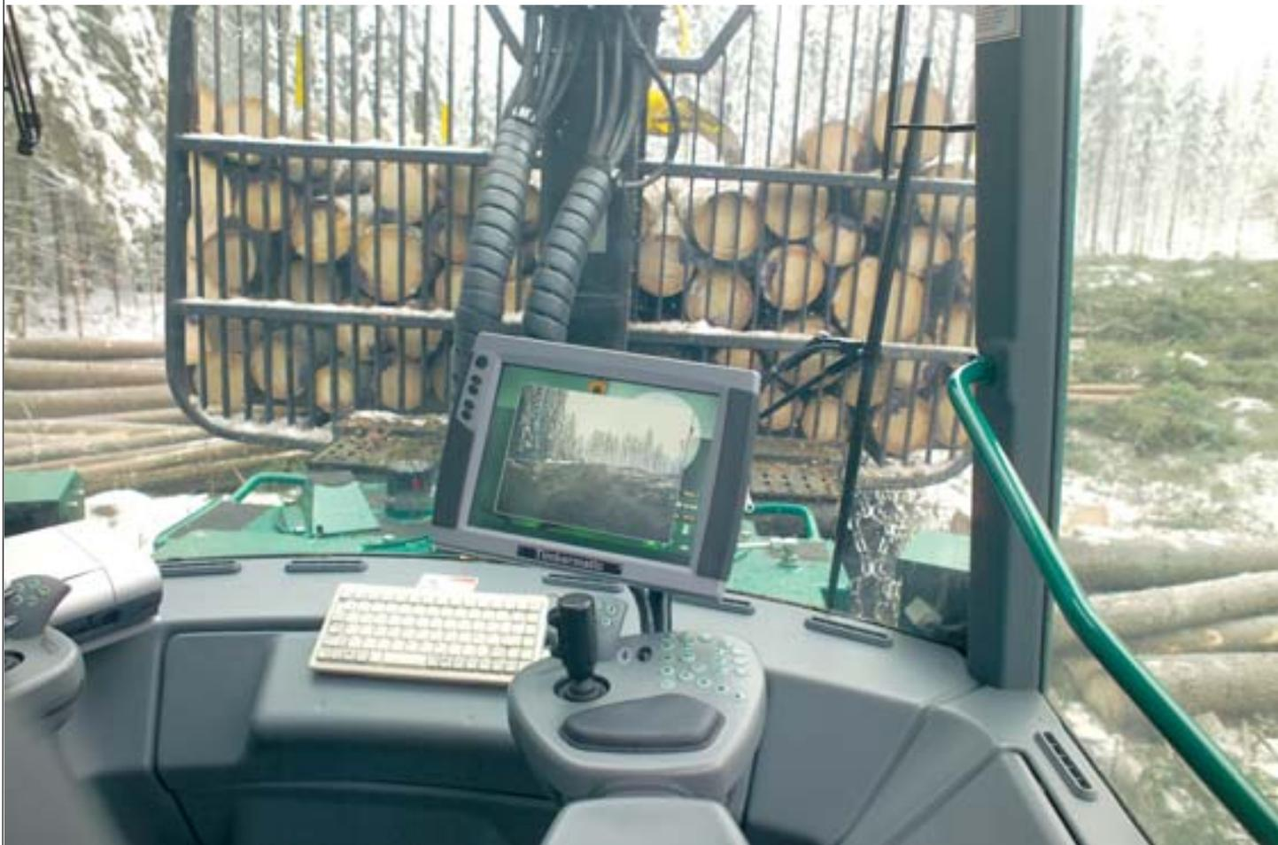
The operator has played a central role in the design of the cab in John Deere forwarders. The cab has excellent visibility, and the sturdy seat and ergonomically designed controls ensure that the operator does not get tired. The comfort of the working environment is further improved by the optional sun blinds, the efficient air conditioning and heating system and the cabin filter, which keeps the interior air of the cab fresh and clean.
