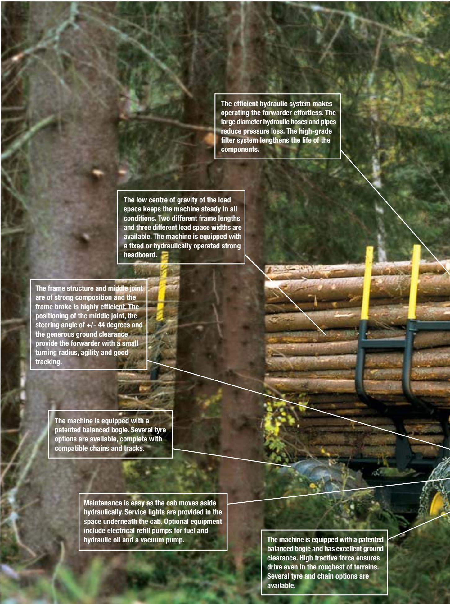
The efficient hydraulic system makes operating the forwarder effortless. The large diameter hydraulic hoses and pipes reduce pressure loss. The high-grade filter system lengthens the life of the components.
