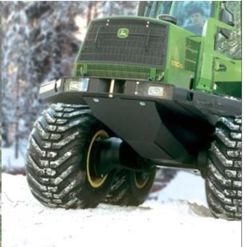
The patented balanced bogie distributes the weight evenly between all wheels. This reduces the ground impact and ensures a gentle ride even when the forwarder is fully loaded.
