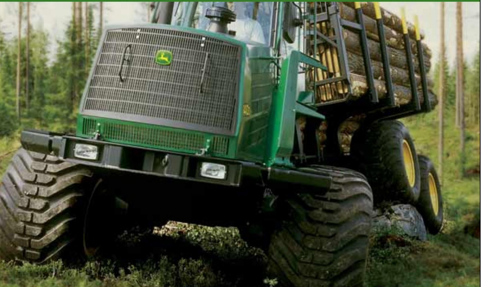
The patented balanced bogie system significantly increases the environmental friendliness of the machine. Evenly distributing the weight between all the wheels reduces the ground impact and provides a smooth ride, even when the forwarder is fully loaded.
