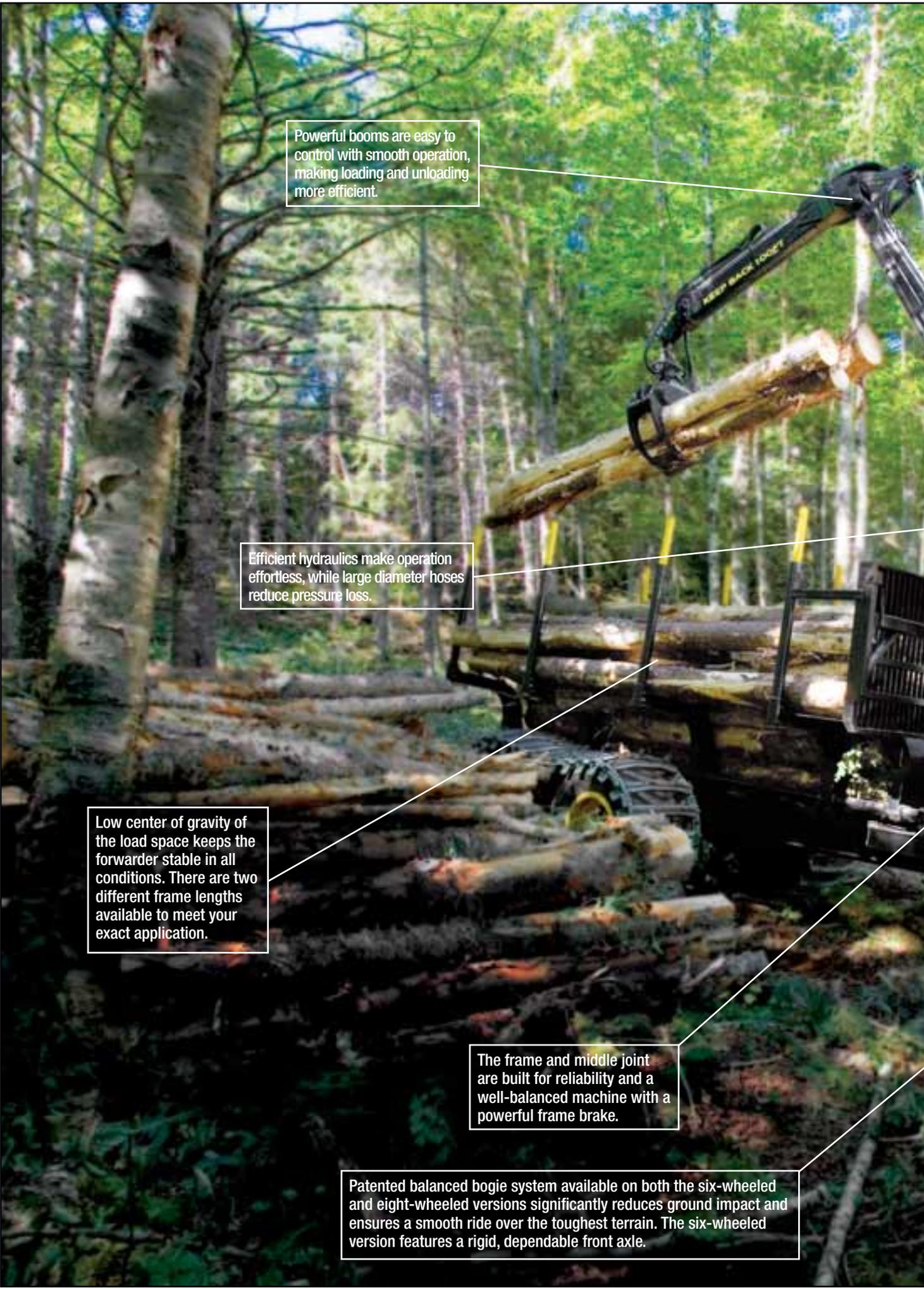
Powerful booms are easy to control with smooth operation, making loading and unloading more efficient.
