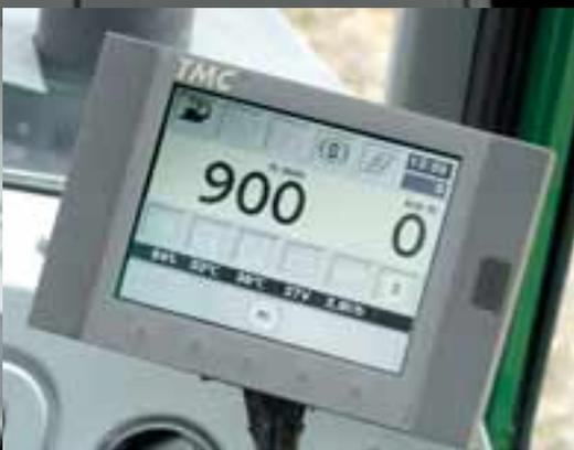
TMC provides valuable information on the different machine functions, such as average or momentary fuel consumption.
