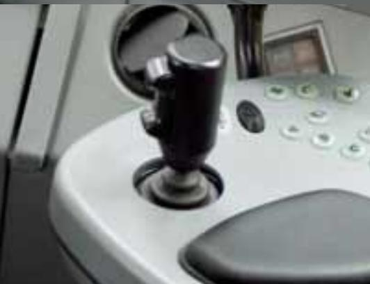
The mini-lever joystick controls mounted on the armrest give you precise control of all loader functions.
