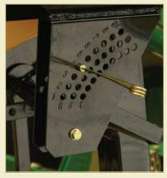
Make simple adjustments to your discharge rate by changing the settings on the spreader rate control. Move the pin higher to increase flow rate or lower to decrease flow rate.
