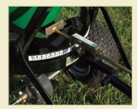
A swath control lever lets you choose either a row or broadcast spread, while also varying the direction of the pattern.
