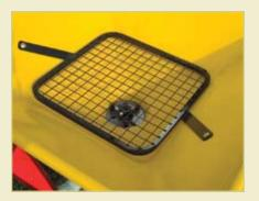
The filter grate (optional) helps prevent clods and foreign material from entering the chute. (SS11 & SS12 Series only.)
