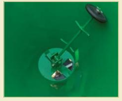
Optional wheel agitator keeps material from packing and bridging over the discharge.
