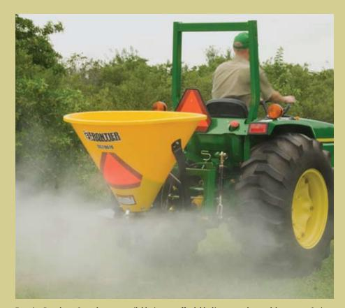
Frontier Broadcast Spreaders are available in two affordable lineups – the steel-hopper 10 Series and the polyethylene-hopper 20 Series. With a capacity range of 3.5 to 10.6 cubic feet and a spread distance of 20 to 46 feet, you get reliable, versatile performance to meet all your spreading needs.
