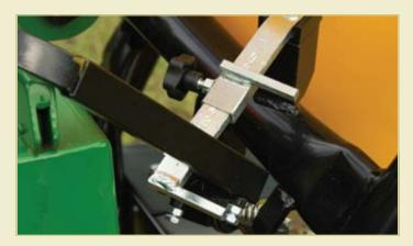
The feed rate lever is conveniently operated from the driver's seat to open the spreader gate when dropping seed and fertilizer.
