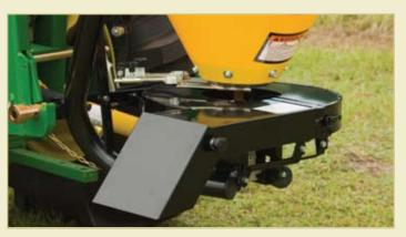
The siderow discharge deflector *(optional)* is easily adjusted to give you improved accuracy and control during discharge.
