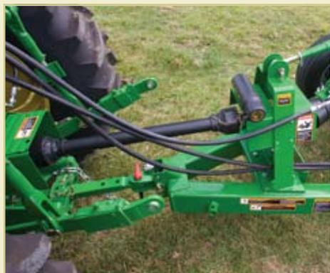
Adjustable height clevis allows the caddy to be leveled to fit the specifics of your tractor, ensuring proper raising and lowering of disc mower.
