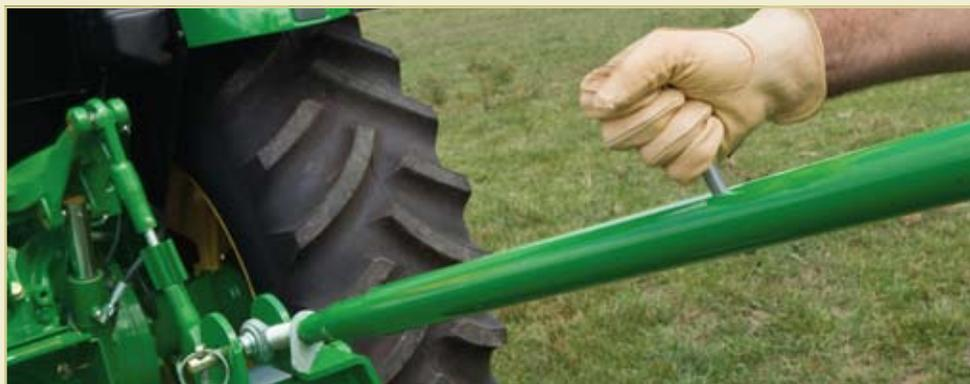
Set cutter depth with the manual turnbuckle adjustment. Shorten the turnbuckle to reduce cutting height. Or for higher cutting height, increase turnbuckle length.
