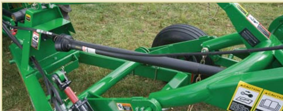
Hydraulic lift rockshaft lets you lower and raise your disc mower from the tractor seat. Transport lock-up bracket prevents your disc mower from lowering during transport, avoiding potential damage to the implement.
