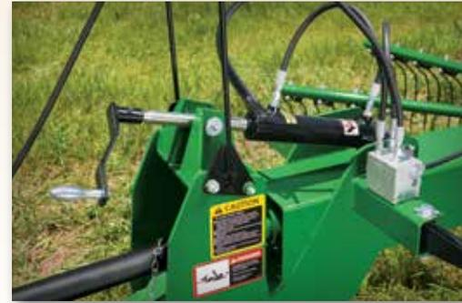
Use the rake-leveling cylinder to set the rake's tine height and pitch. This adjustment allows you to fine-tune ground-pressure in a variety of crops and conditions.
