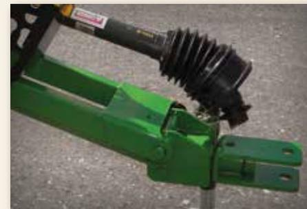
Standard clevis hitch-link allows you to easily connect to your tractor. Safety chain comes standard.
