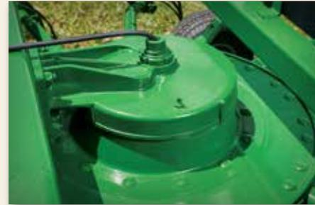
Frontier Rotary Rakes are equipped with a fully enclosed gearbox to keep dirt, debris, or hay from getting inside. It allows for improved reliability, and includes oil bath lubrication for increased cooling.
