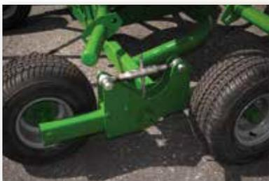
Tandem-axle walking beam keeps the rake level over uneven terrain to provide a smoother ride and to promote better crop pickup. And four large flotation tires offer added stability over rough fields. Four additional flotation tires are optional on the RR2324 to give you level raking performance on contours and over uneven ground.
