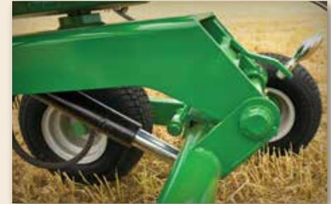
The RR2109, features a rear height-adjustment screw that lets you set the height of the tines for optimal performance in a variety of crop conditions.
