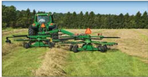
One window or two? The RR2324 Tandem makes the decision simple. Just choose the double- or single-window option to adjust the twin rotors, and then set the desired window width.
