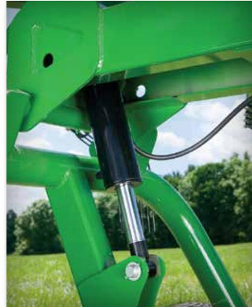
The hydraulic lift allows you to raise or lower the rake for transport. Generous under-frame clearance prevents windrow damage when turning around in the field.
