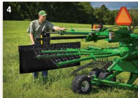
**(1)** An adjustable, heavy-duty vinyl curtain on the RR2109 and RR2211 helps maintain consistent window width. Remove the curtain to combine multiple windows. **(2)** An easy-to-use hand lever on the RR23 Series offers fast, simple control of window width. **(3)** When using the RR2324 Tandem Rotary Rake, the rear curtain can be adjusted hydraulically to vary window width. **(4)** And the rear curtain on the RR2324 can also be adjusted with a pull of a lever for quicker transport.
