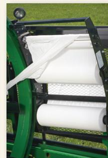
Get twice as much wrapping with a twin wrap kit. Double wrapping helps reduce puncturing when working with straw or dry hay.
