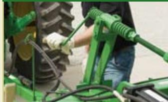
Easy hand crank lets you adjust the disk fore-and-aft, ensuring level disking performance.
