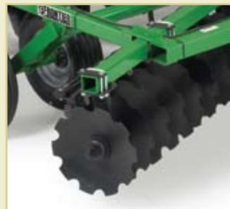
The DH16 Series offer two types of blades: notched for aggressive cutting and increased penetration, or smooth for a clean slice when sizing and mixing residue. Use a single style blade or go with a combination of both.
