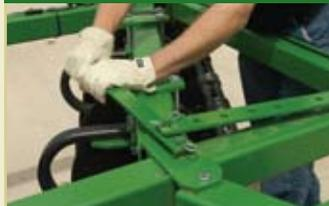
For lighter soils and low residue levels, simply reduce the angle to turnout picture-perfect seedbeds.
