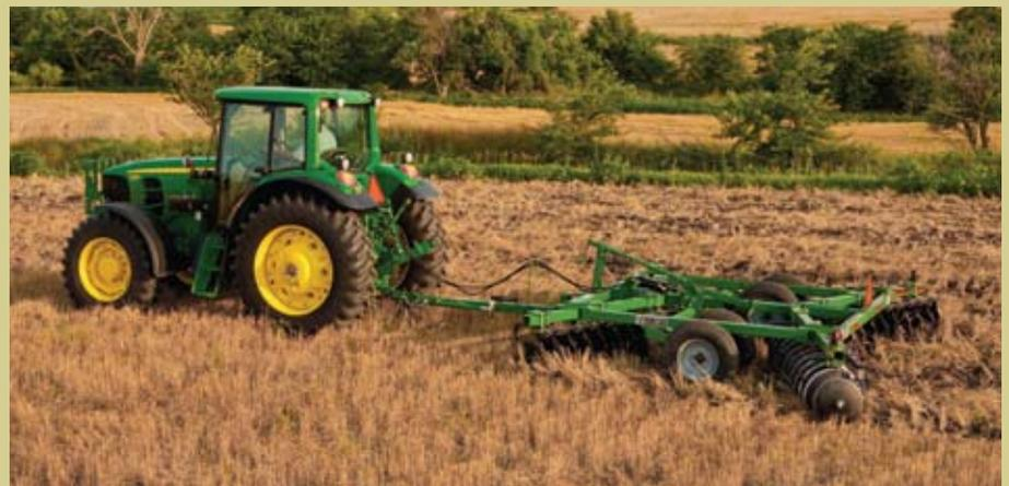
The DH16 Series cuts through heavy corn stalk, thick wheat stubble, tough sod, and more. Adjustable front and rear gang angles let you bury the amount of surface residue to meet your needs.
