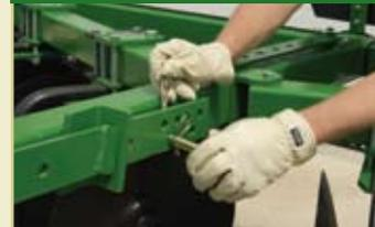
A convenient adjustment pin lets you set depth, fast and easy, and maintains that depth on every pass – so you don't have to worry about cylinder donuts.
