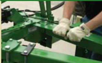
Independent front and rear gang angle is easily adjusted to handle a variety of soil conditions. Just increase the angle for more aggressive disking when working in heavy residue.
