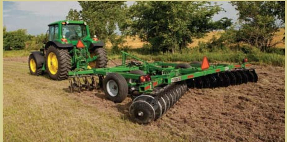
You know you're working with heavy-duty machinery when you hook up a Frontier DH16 Series disk to your tractor. A sturdy frame, 22-inch-diameter and .177 inch thick steel blades, and a commanding 130 pounds of weight-per-blade provide excellent penetration in heavy residue and hard ground.
