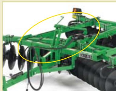
A level-lift hitch provides more-consistent tillage depth when working uneven terrain, and keeps the disk level when making minor depth adjustments, or when raising the machine out of the ground during transport.
