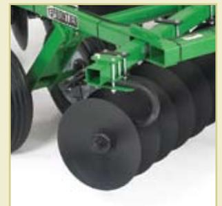
Got rocky fields? The DH16 Series can also be equipped with optional C-spring gang hangers to lessen the shock load and optional .236 inch blades for greater durability when working over rocks and debris.
