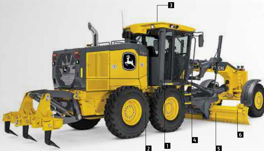
**1** Exclusive **Auto-Shift PLUS** – also available on all G-Series models – allows operators to work without using the inching pedal.
