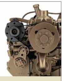
It all starts with the turbocharged diesel John Deere Tier II 6081H engine that generates more power than most compact machines. This powerhouse delivers steeper torque rise, producing 5% more horsepower at 2,000 rpm, and 5% more torque than engines used in previous models. It's quieter, too, with isolation mounting and low restriction mufflers.
