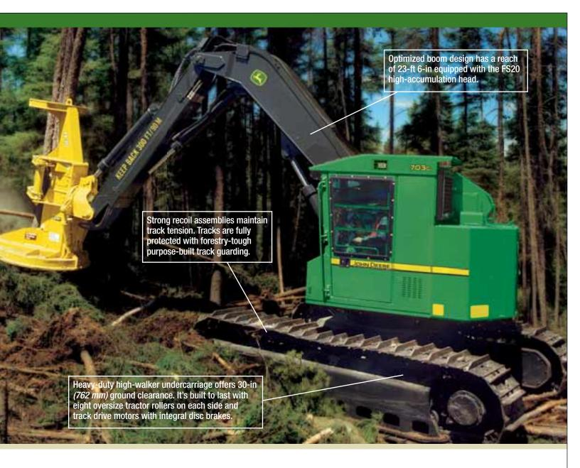
Whether final or selective cutting, the 703G is "heads" above the competition. For selective cutting, its almost zero-tail-swing over the back allows you to weave your way into dense stands and still have room for boom maneuverability. For big bunches of small stems or large timber, the 703G has lots of power and hydraulic strength to handle the load. The powerful boom set and sturdy lift capacity at full reach are all designed to keep you in the field, and keep your business in the black.
