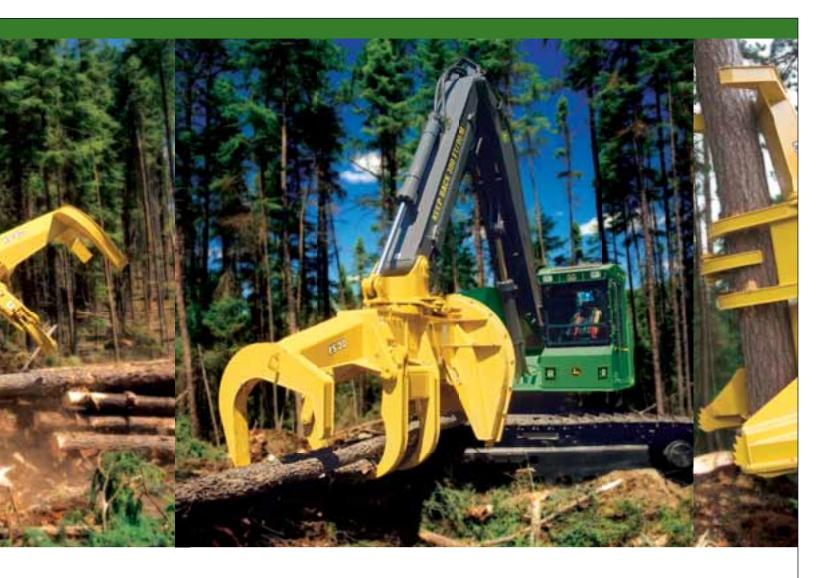
With its large footprint and low center of gravity, the 753G offers incredible stability and low ground pressure from "roll-up."
