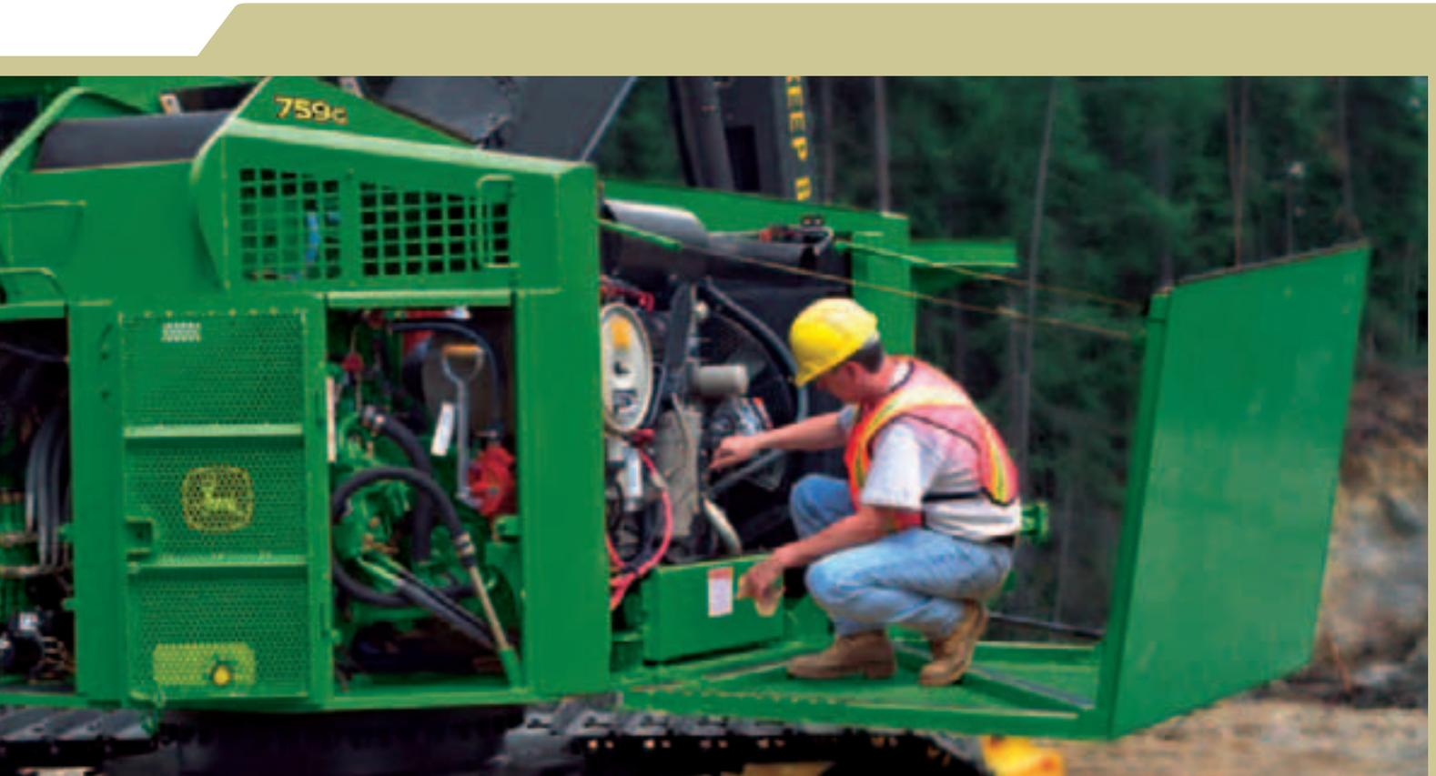
Debris clean-out and scheduled servicing is faster with the hydraulically opened engine enclosure and easier with work platform access.
