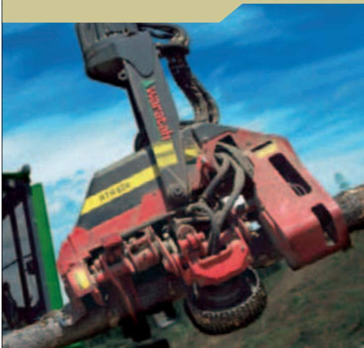
The HTH620 is ideal for applications where 80% of the trees are 16-in. (40 cm) in diameter or less. Highly productive in thinning or regenerative harvesting in both hardwood and large diameter softwood.
