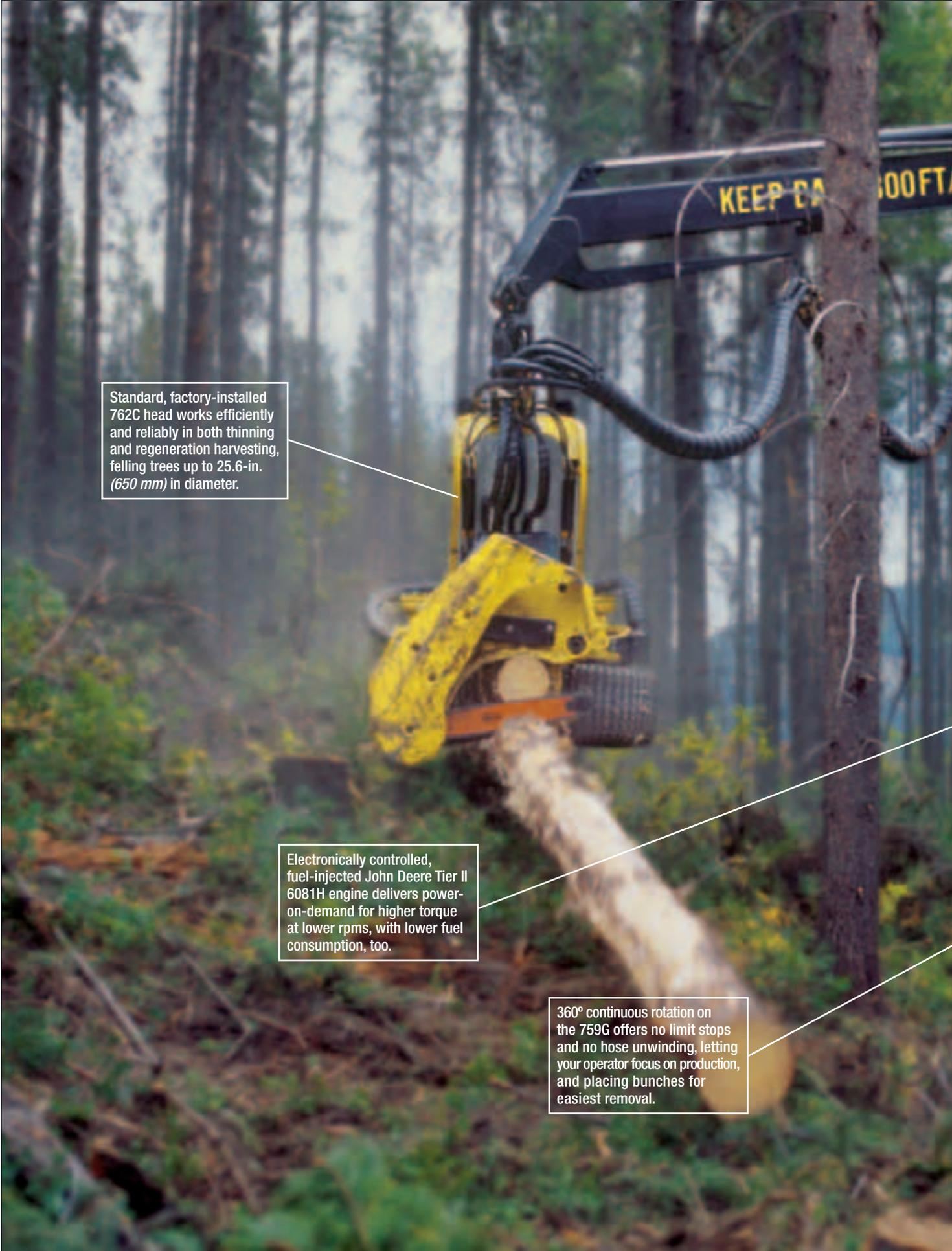
Standard, factory-installed 762C head works efficiently and reliably in both thinning and regeneration harvesting, felling trees up to 25.6-in. (650 mm) in diameter.
