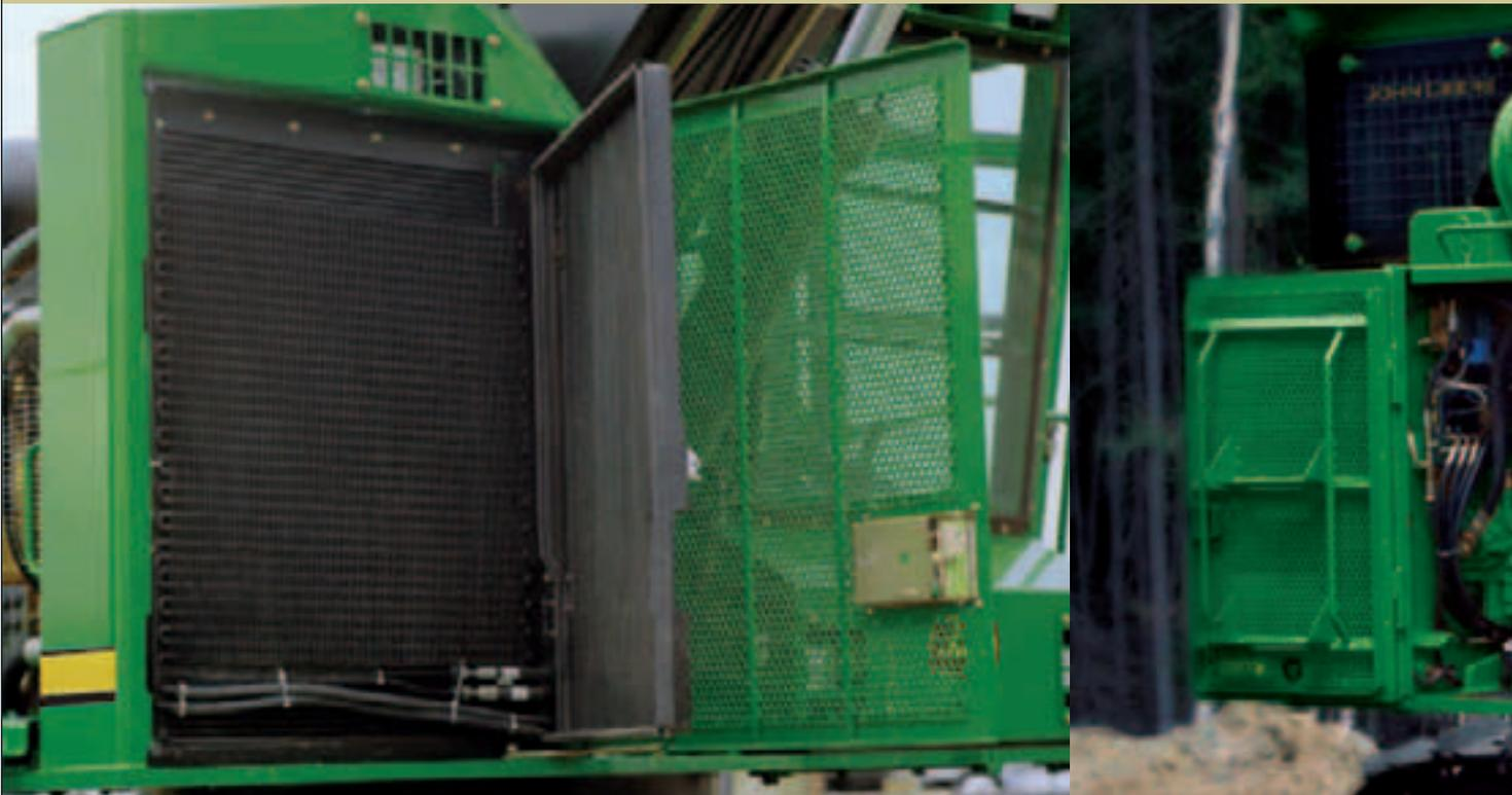
An optional reversible fan purges debris from coolers, which extends the engine's life and makes it run more efficiently.
