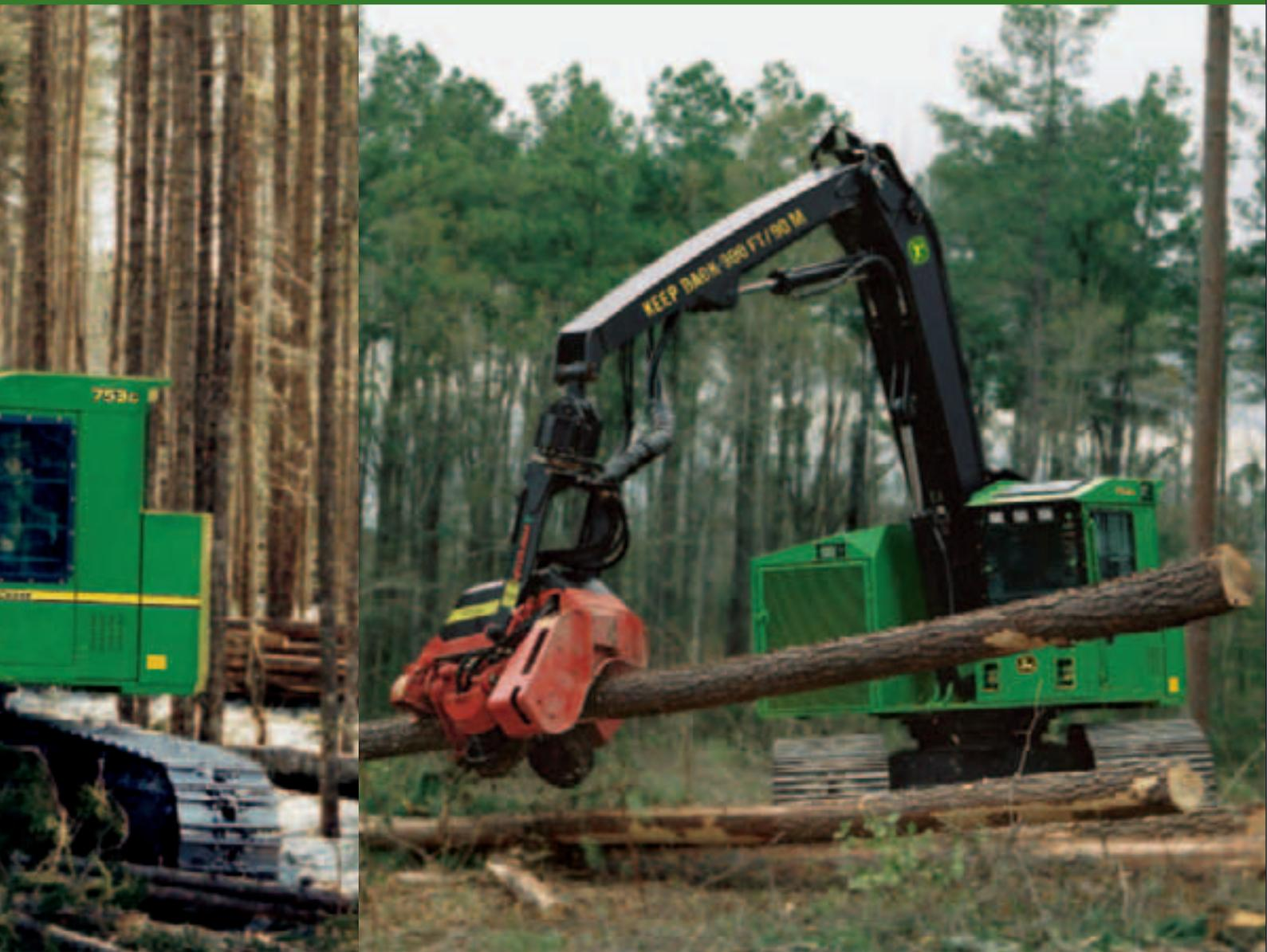
Near-zero tail-swing over the rear with only 10-in. (250 mm) over the side of standard tracks.
