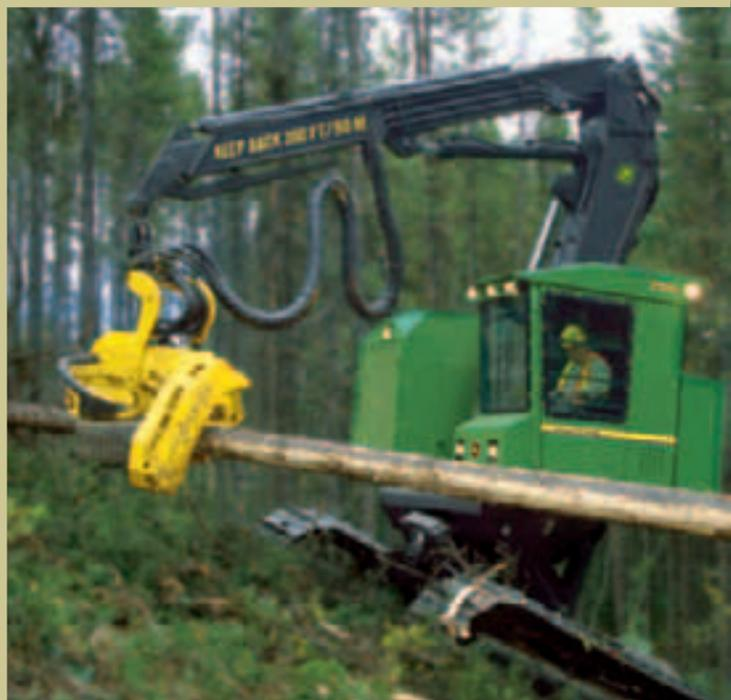
27-in (685 mm) saw bar on the 762C automatically extends only far enough to complete the cut, reducing the chance for damage while felling. Powerful feed rollers handle the tree gently, and superior delimiting is handled with four moving and two fixed delimiting knives.
