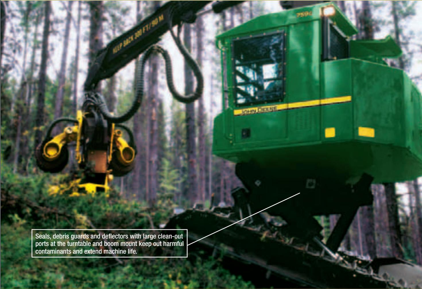
Seals, debris guards and deflectors with large clean-out ports at the turntable and boom mount keep out harmful contaminants and extend machine life.
