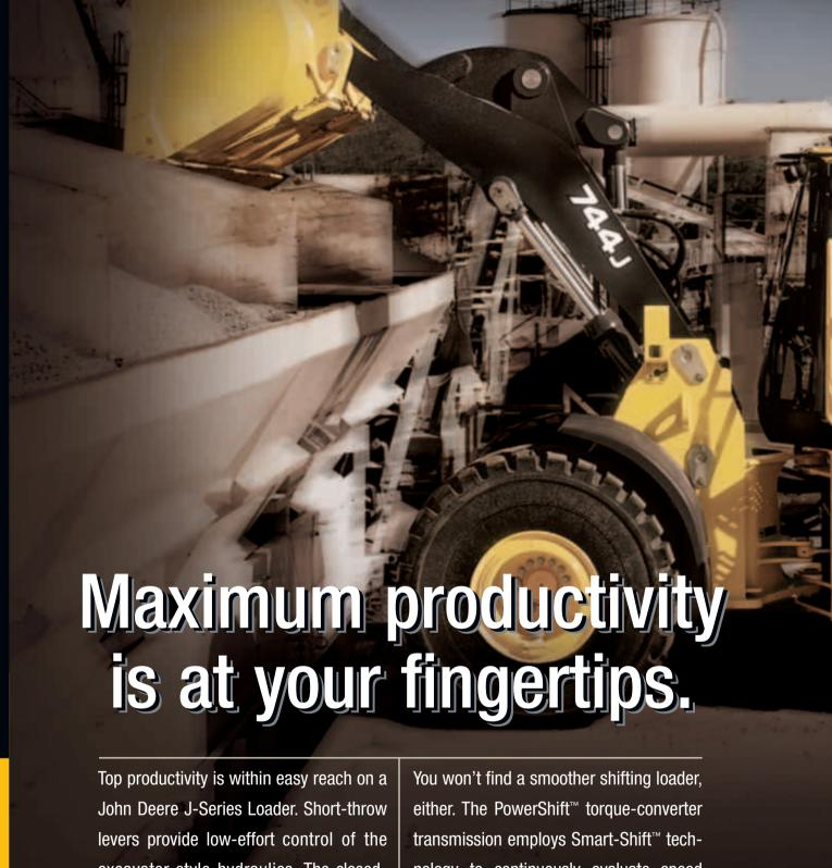
excavator-style hydraulics. The closedcenter system senses the load and delivers the power needed for smooth boom and bucket functions and fast cycles.
