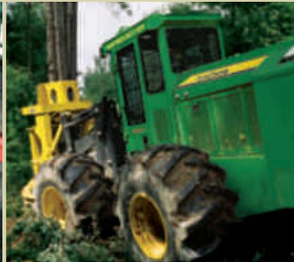
Parallel geometry of the arms and linkages keep trees vertical when the boom is raised.
