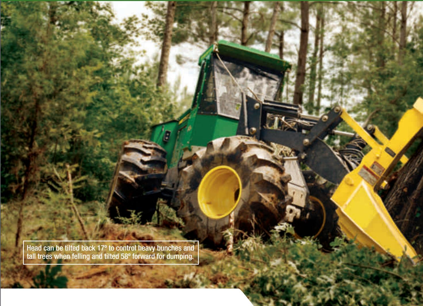
Head can be tilted back 17° to control heavy bunches and tall trees when felling and tilted 58° forward for dumping.
