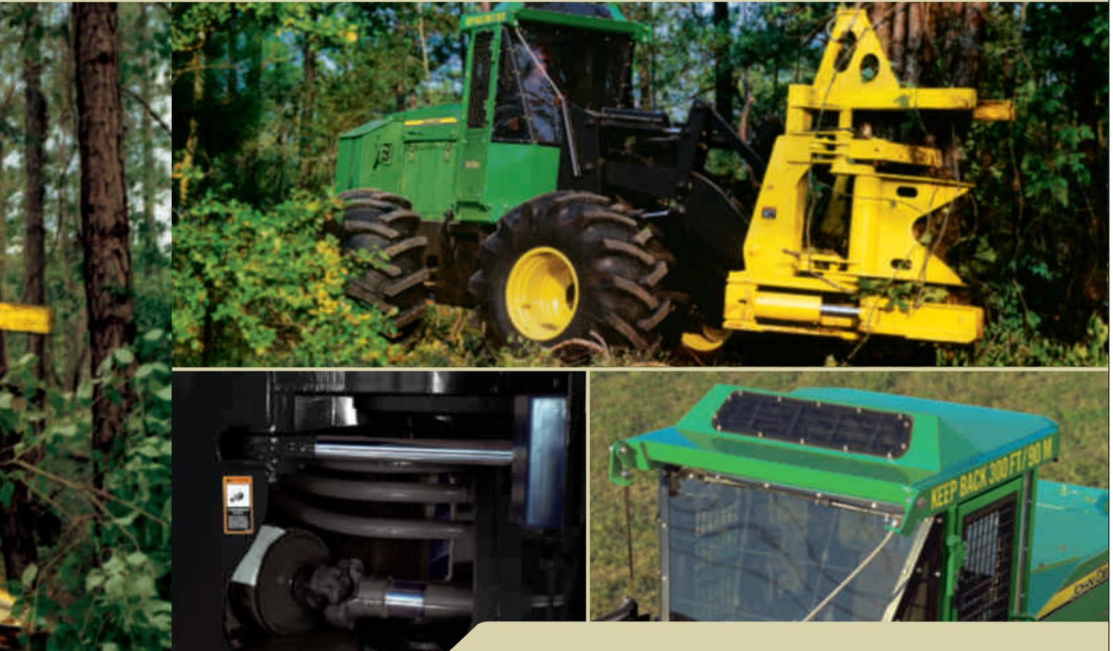
Strong center hinge with large tapered roller bearings give long-life reliability to this critical area.
