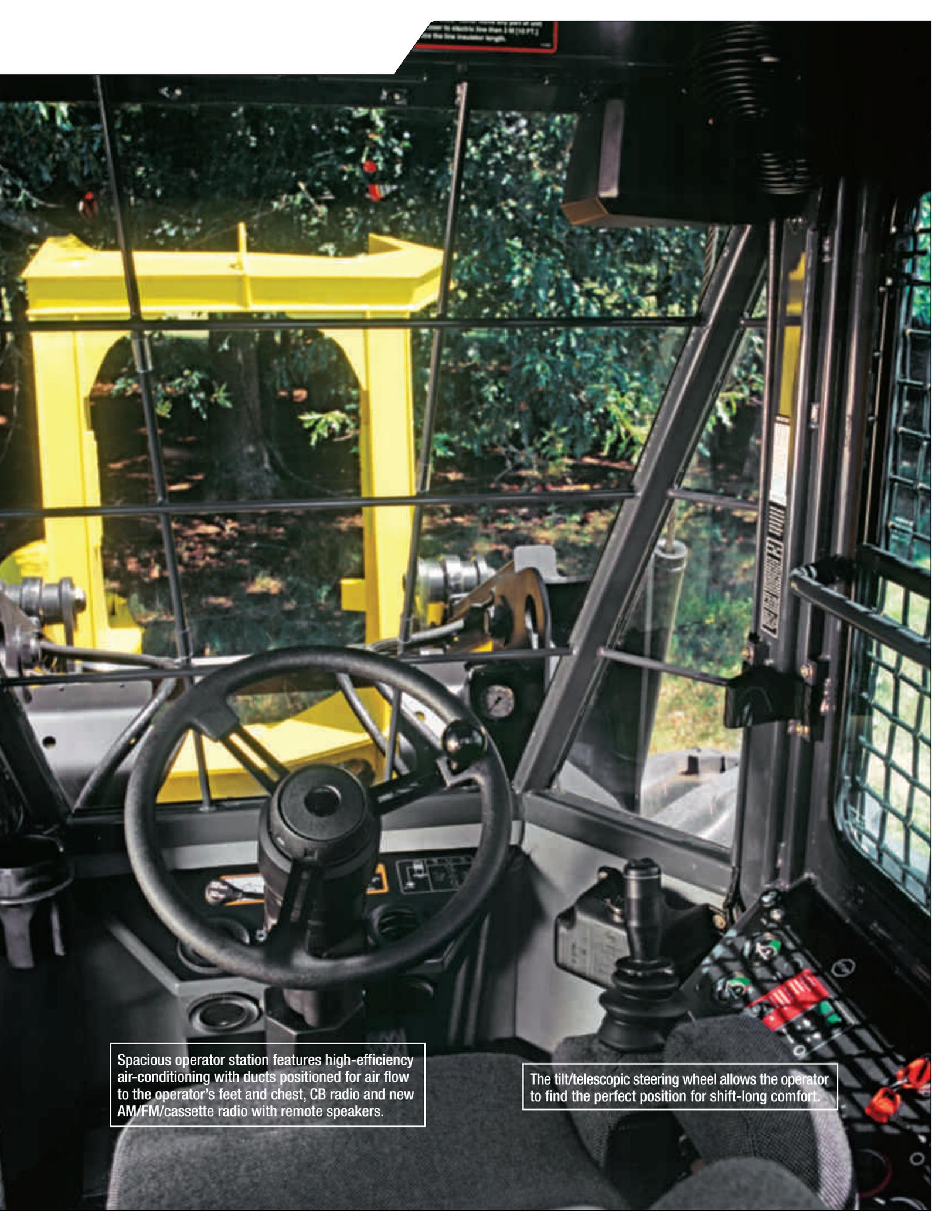
Spacious operator station features high-efficiency air-conditioning with ducts positioned for air flow to the operator's feet and chest, CB radio and new AM/FM/cassette radio with remote speakers.
