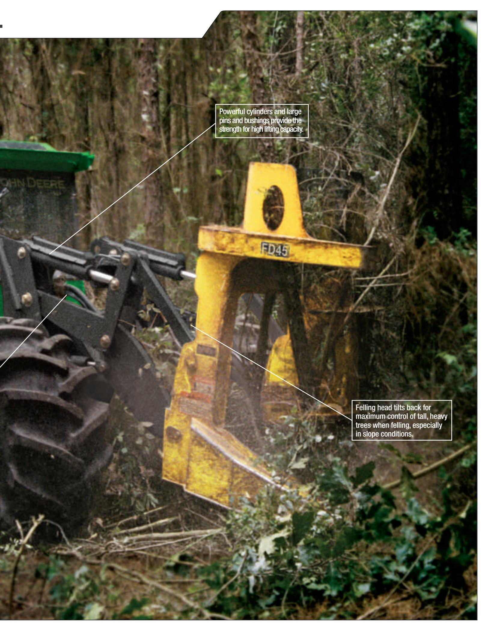
Powerful cylinders and large pins and bushings provide the strength for high lifting capacity.
