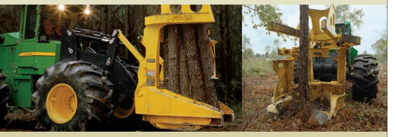
The FD45 felling head has best-in-class size and productivity, with an offset pocket to gather multiple small stems. Single-side accumulating and gathering arms reliably gather and move stems to the pocket cut after cut. The twin-post design gives the operator a clear view of what he's cutting.
