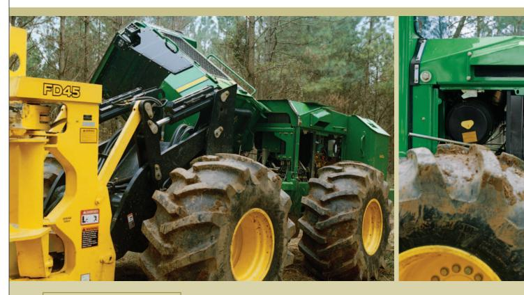
The J-Series features best-in-class serviceability access with a tilt cab and full-service access panels. The air cleaner assembly is angled for easy replacement.
