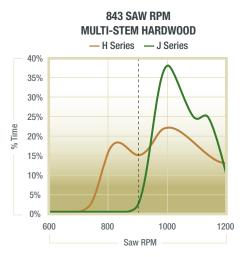
When it comes to production, it's all about time. And your time should be spent cutting, not waiting. To cut effectively, the saw speed should stay above an average speed of 900 rpm (depending on the application). The new J Series, with increased horsepower and power management, can maintain higher saw speeds for longer periods of time, even in demanding hardwood applications. Simply stated, the saw is available to cut more often, resulting in a significant productivity increase.
