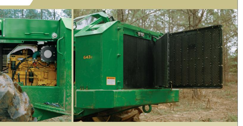
The heavy-duty rear grill has been designed to filter out fine particles before they get to the coolers and cause big problems. The swing-out design makes for easy access.
