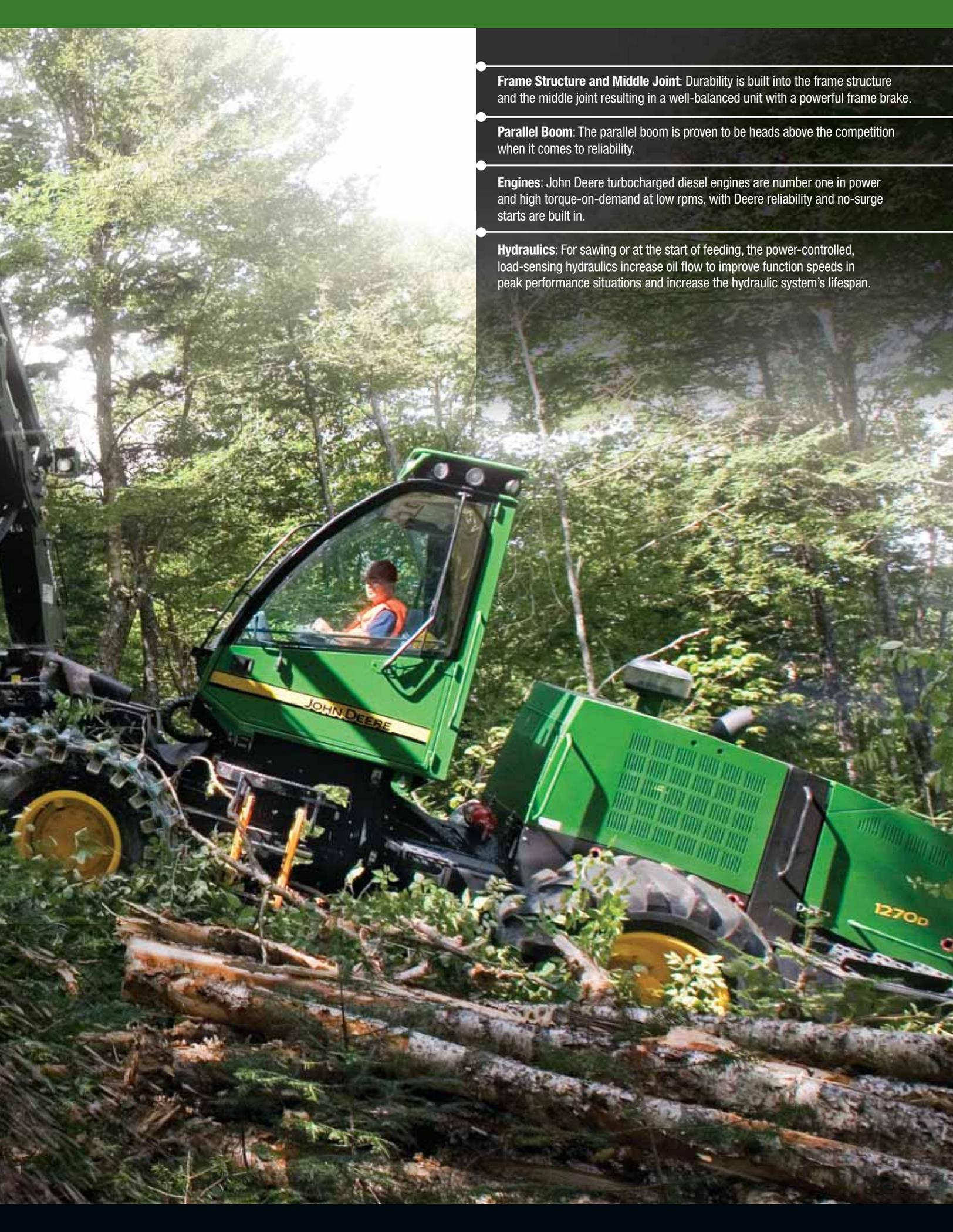
**Frame Structure and Middle Joint:** Durability is built into the frame structure and the middle joint resulting in a well-balanced unit with a powerful frame brake.
