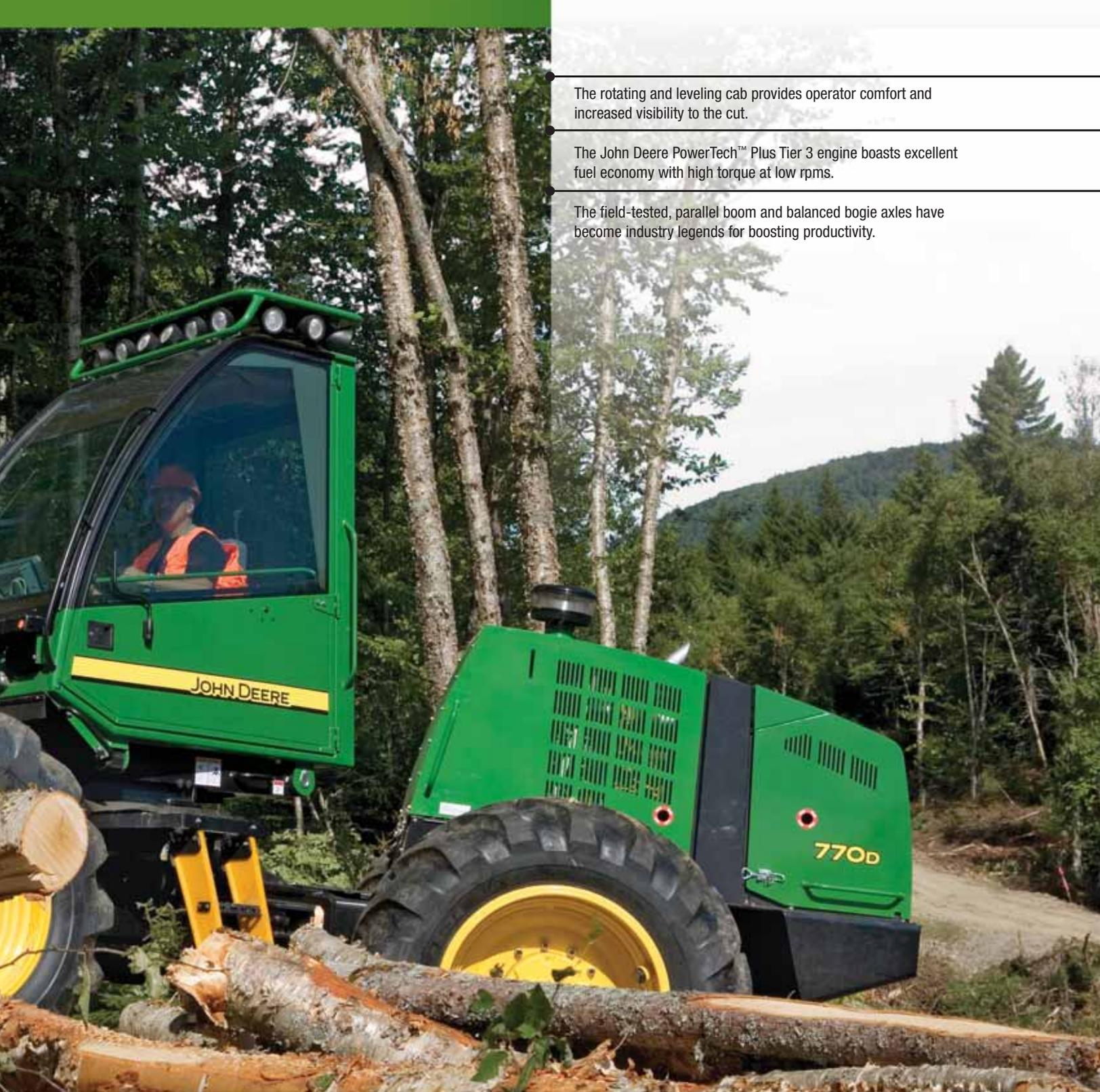
The rotating and leveling cab provides operator comfort and increased visibility to the cut.
