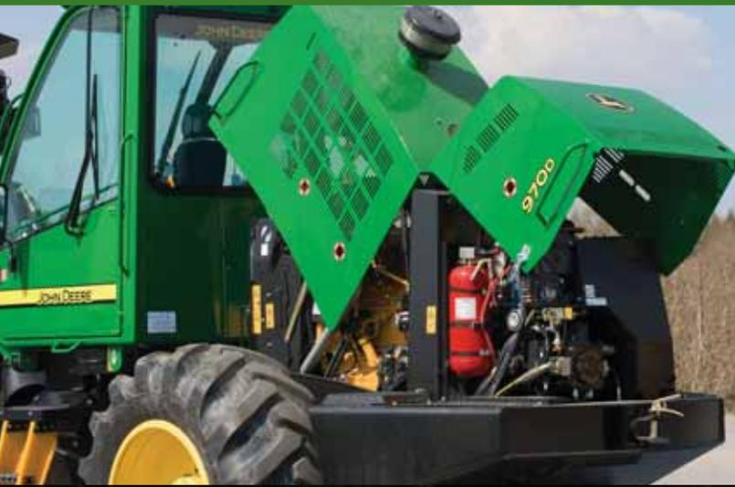
**Easy Safe Maintenance Access:** For easy maintenance, the engine hood is comprised of two sections and is operated by an electrical motor for easy access.
