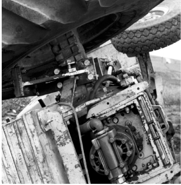
Following each rollover test, engineers took dozens of pictures to ensure that the welds and bolts could stand the stress. This photo was taken in September of 1963.
