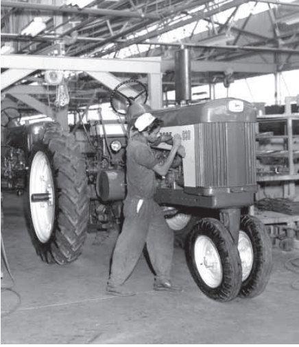
Monterrey, Mexico's John Deere plant built the versatile 630 Row Crop Tractor, like the 1959 model shown at left. Each was powered by a 5.0L, 2-cylinder gasoline, all-fuel, or LP-gas engine.
