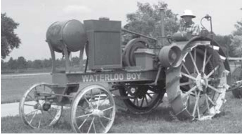
The Waterloo Boy Model "N" was powered by a traction engine and had a 2-speed transmission that moved the tractor at 2.3 and 3 mph.
