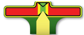
**Critical:** Draper belt tension indicator must be in the position shown to ensure proper draper function in all conditions.
