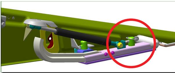
Also, ensure storage pin is placed in correct location highlighted above.
