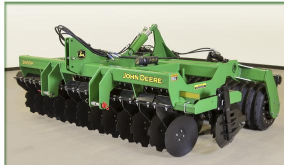
**IMPORTANT:** Do not reverse machine in ground or damage may occur. Activate tractor 3 pt hitch lock (if equipped) when transporting.
