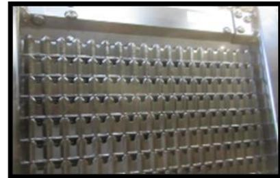
Be sure chaffer and sieve are calibrated so the opening exactly matches the cab display setting.
