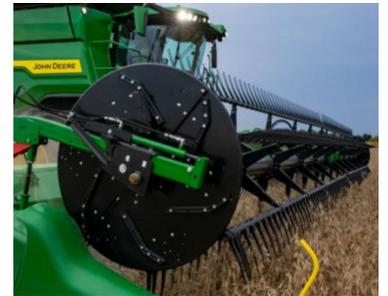
**Gauge Wheel Scrapers** Recommended to reduce gauge wheels from accumulating material which could cause inaccurate header height position for off-ground cutting. (*Gauge wheels only available on HD*)
