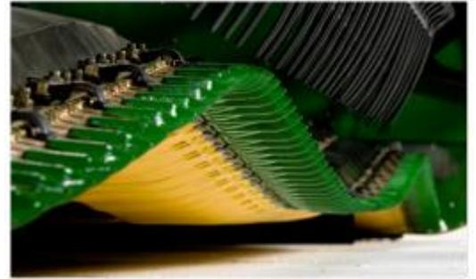
**HDR:** With the wings in the down, measure 45mm at the outer reel fingers and 15mm at hinge.
