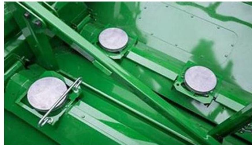
*ActiveYield force sensors within the grain tank.*
