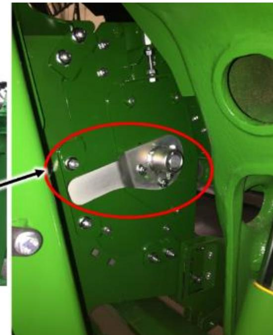
Rotate handle clockwise to make the fingers more aggressive. More aggressive finger timing is recommended for low volume crops such as dryland wheat, lentils, and flax.
