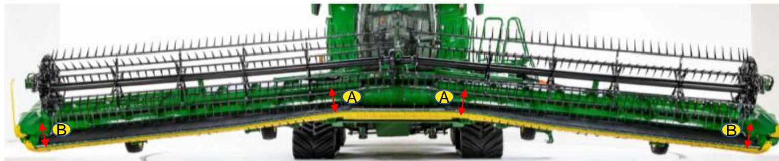
Note: It is acceptable if reel fingers to contact the crop ramps (A) during a full frown state. This setting will allow for reel fingers to perform best in the flat position.
