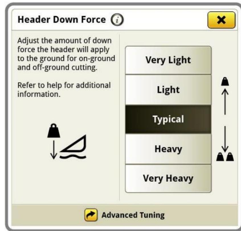
*The advanced tuning page should only be used in extreme conditions as you can over adjust the head and cause it to perform very poorly*
