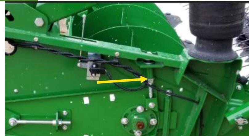
**Without Feed Auger Spacer**
