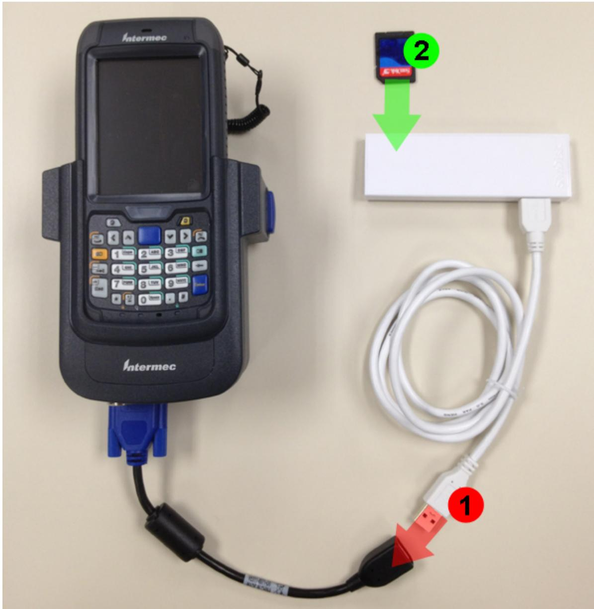
**Connecting the External Memory Device Reader and Memory Device**
