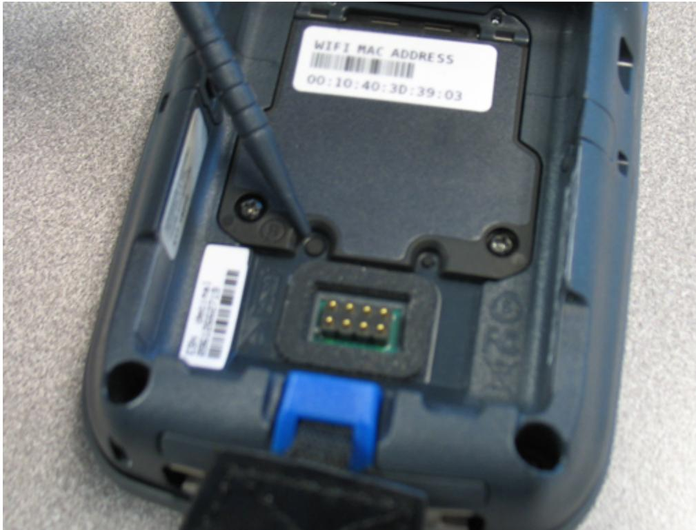
As previously-stated, you can't actually shut most mobile devices off. For an Intermec™ CN70, pressing the "power button" merely pauses the CPU's operation. Power continues to flow to its RAM, so it's ready to resume operation instantly the next time you press that button.
