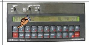
• Press the CE button until 9600 is displayed. Then press the 1 or 2 Arrow buttons until DATA LOG TRIGGER VALUE is displayed.
