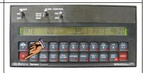
Press the ENTER button and then the number 1 button. Then press the 1 or 2 Arrow buttons until DATA LOG TRIGGER UNITS is displayed.
