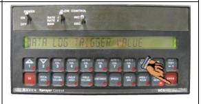
Press the CE button so that SEC is displayed. Then press the 1 or 2 Arrow buttons until DATA LOG is displayed.
