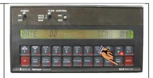
• Press the 1 or 2 Arrow buttons to scroll through the list of items until BAUD RATE is displayed.
